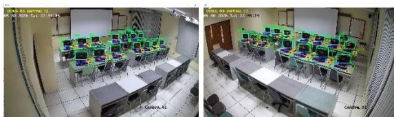
Figure 2. Polygon ROI mapping used in the proposed multi-camera system: (a) primary camera (C1), (b) backup camera (C2), and (c) backup camera (C3).
